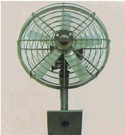
the column. A heavy steel tubular support is provided for mounting the fan. The air stream may be adjusted in horizontal and vertical plane by providing tilting arrangement. Wire-guard is also provided for both sides of the impeller for protection.
